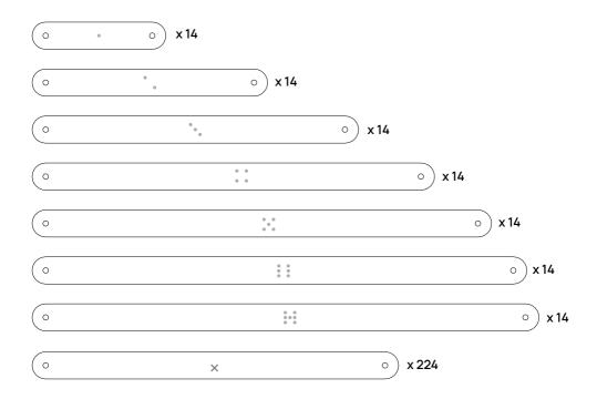
Total: 350 precision manufactured bamboo strips 130 stainless steel nuts and bolts
