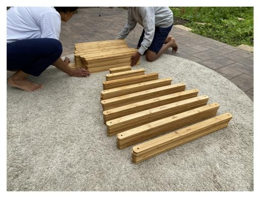
The strips with dots are of varying sizes and go horizontal in the Zome. The strips with X are all the same size and form the diagonals. You can arrange them in order of dots from 1, 2, 3, 4, 5, 6, 7, 6, 5 and will see the shape of the Zome appear.
