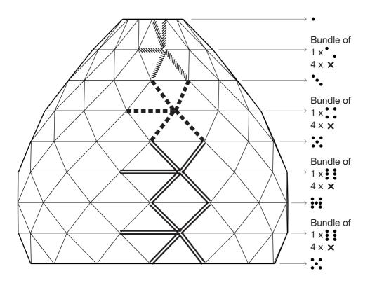
The bundles of 5 strips is arranged in a star shape as per the diagram and connect to the adjoining bundles on the side.
